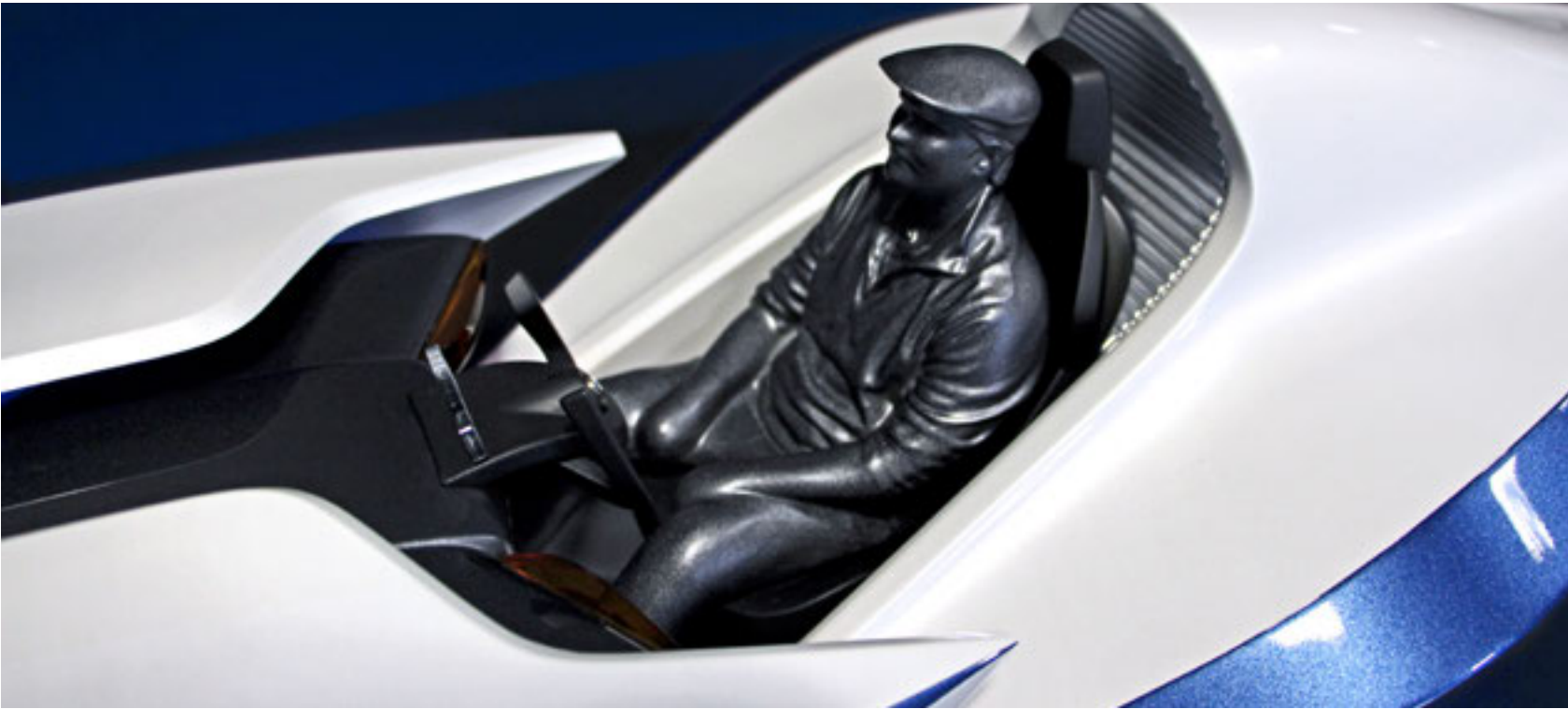
3D Printed Driver & Air-Intake
